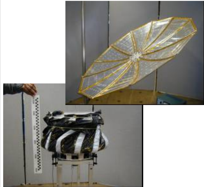
Collapsible Ribs Tensioned Surface (DSL Cambridge University, ESA patent)
